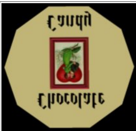
Fig. 2_21 Normals wrong, texture mapped incorrectly.
